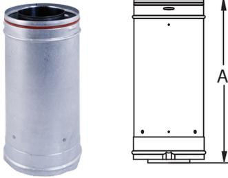
Features fully unitized, twist-lock construction in 3" diameters. It can be used in both vertical and horizontal installations. Stainless steel welded seam inner wall, combined with a galvalume welded seam outer wall. Inner and outer are sealed with O-Ring gaskets. Galvalume or painted black outer finish. To calculate installed length, subtract 1 1/2" from each length of pipe.
