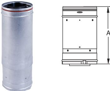
Use to add length to straight lengths of CVS pipe. Amount of adjustable length listed in chart. Requires at least 1/2" overlap for a secure connection.
