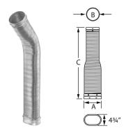
Use through damper and smoke shelf area. Use to connect from oval stove outlet to round DuraLiner. Use with DuraLiner Insulation Kit (ProMesh and ProFoil), where flex extends into clay liner, for zero-clearance applications. Built from 1-ply construction, .005" 304 stainless steel.
