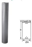
Use to reline masonry chimney with 0/0 clearance. Factory-insulated. Twist-lock fittings and pre-drilled hole (one screw required). UL Listed for zero clearance between masonry and combustibles, plus zero clearance between liner and masonry. 304 stainless steel inner and aluminized steel outer. Note: to calculate the installed length of 5", 6", and 8" DuraLiner pipe subtract 1 ½" from each joint overlap of liner pipe sections.
