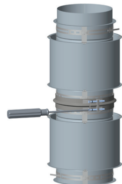
Figure 9 - Joint Assembly Step 4
