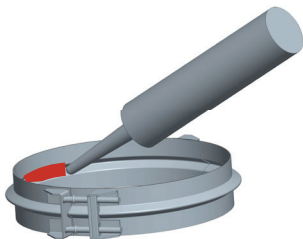
Figure 6 - Joint Assembly Step 1
