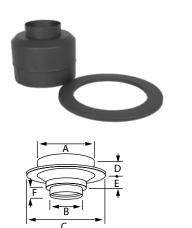
Identical to the DTC-FSC Round Finishing Support except this version has a removable trim collar. This allows collar to be fastened in place after finish of ceiling is completed. Integrated adapter accepts either single-wall or double-wall stovepipe.
