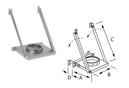
Use to support insulated tee on though-wall chimney installation. Access for inspection and service is incorporated from the underside of this support. Adjustable arms and sliding base plate are factory-set to ensure minimum clearance of 2". Allows for 2" - 7" clearance to combustibles.
