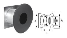
Designed to protect surrounding combustible materials in throughthe-wall installations. Trimmable thimble can accommodate wall thicknesses from 7" up to 12-1/2". Includes wide, decorative trim collar for professional finish. Thimble is fully Insulated to minimize heat-loss and cold air intrusion.
