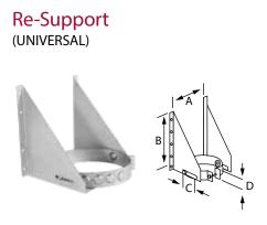
Use to support the chimney on a vertical wall. The triangular plates allow for a 2 <sup>3</sup>/<sub>4</sub>" adjustment of the support to the vertical surface. This support can also be used as a wall support above the insulated tee or as a support for an offset elbow. Refer to chart for load bearing capacity. In shorter chimney stack applications, the Re-Support can also be used in place of a Tee Support. Universal design works with 6", 7", or 8" pipe diameters.
