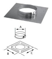
Use to support the chimney on a slab, floor, or joist and also acts as a firestop. It includes a tightening collar that locks around the chimney and is secured by self-tapping screws (included). The collar rests on a horizontal plate screwed or nailed to the floor or slab. It can also serve as an intermediate support. Refer to chart for load bearing capacity.
