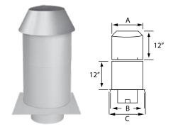
Two-piece telescoping shield adjusts from 12" up to 22" height to accommodate deeper insulation. Shield is insulated, and comes with collar shown.
