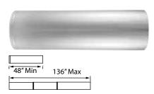
The rigid shield includes three overlapping sections that telescope to match required ceiling height. The bottom rests within the ceiling support for the chimney below. The top attaches to the bottom of the Radiation Shield Connector above. See installation instructions for more information.
