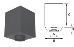
Support for use with vaulted or cathedral ceilings. 6" version fits within 12" x 12" frame. Larger 7" and 8" versions will fit within frame between 16"-on-centre construction. Includes two-piece adjustable black finish trim. Integrated adapter accepts both single-wall or double-wall stovepipe.
