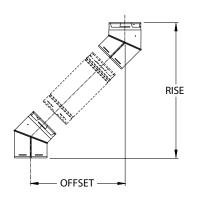
Use to determine the lengths required for an installation. Determine the offset required in view of the obstacles that must be avoided. Refer to the offset/rise chart to determine the elbows required as well as the insulated lengths needed. Check the corresponding offset height dimensions.
