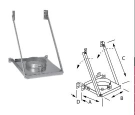
Use to support insulated tee on though-wall chimney installation For installation versatility and convenience, tee can be placed above or below the support. Must be paired with twist-lock tee cap. Can also be used as a wall support or re-support. Adjustable arms and sliding base plate are factory-set to ensure minimum clearance of 2". Allows for 2" - 7" clearance to combustibles.
