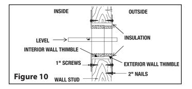
Step 3. The minimum length of insulated chimney required to pass through the wall will be wall thickness plus 7". The insulated chimney must extend at least 5" into the room beyond the finished wall. Insert this chimney length in the side branch of the insulated tee. Turn it clockwise to lock it in place. Seal this joint by wrapping it with the aluminum tape supplied with the tee.
